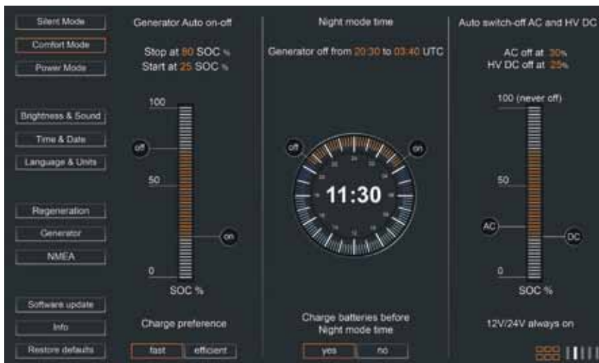
Settings category: Comprehensive and easy to operate menu. Customize displays with your preferred settings and explore options like night mode, which ensures batteries are fully charged by a specified time and can provide power without generator noise.
